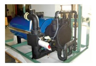
llustration of tank and evaporator for cooling mediums -40°C being prepared for international engine test standards for international automakers.
