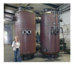
Tanks with 12,000 litres and four dual-circuit evaporators, connected to 8 refrigeration systems, for the catering company of Emirates, Dubai airport. A similar plant has been installed in Frankfurt for the catering company – Lufthansa Sky Chefs.
